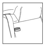
3 Lower the seatback(s) by pulling forward on the tab located on the outboard side of the seatback(s).
